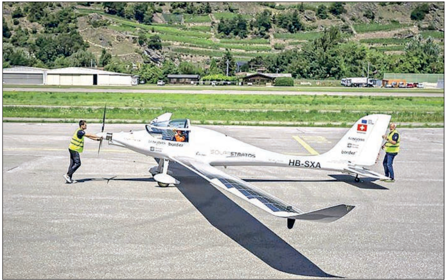
The SolarStratos plane has 22 square metres of solar panels on its wings. PHOTO: AFP
