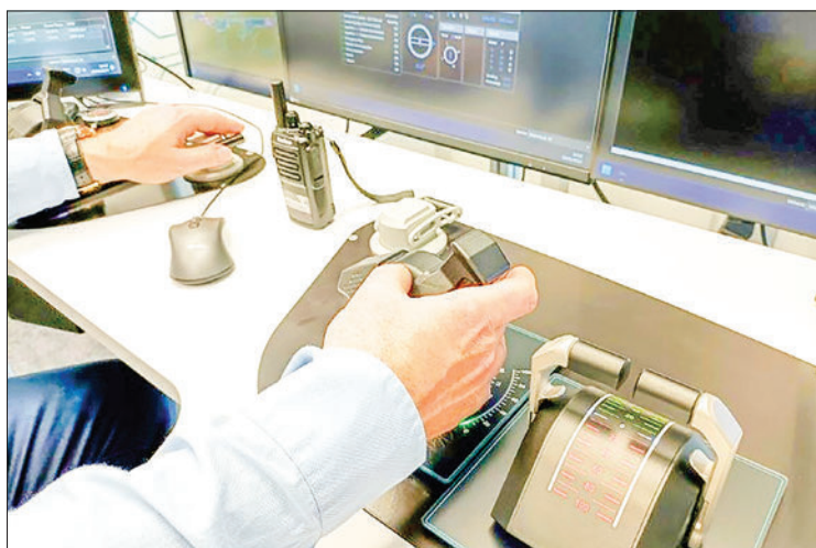
HGK Shipping, based in the German port of Duisburg, is testing a plan to navigate its vessels remotely from a control centre on land. PHOTO: AFP
