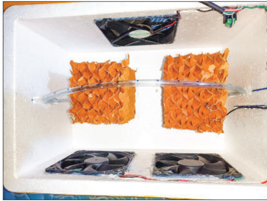
Clothing bin air cooler innovated by Ko Win Moe Kyaw.
