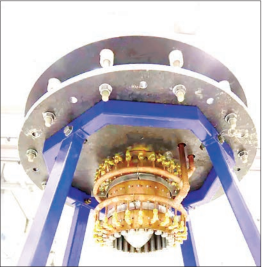
The image shows a laboratory prototype of a plasma electric rocket engine developed by Russian scientists at Rosatom. PHOTO: REPRESENTATIVE IMAGE / SPACE INSIDER
